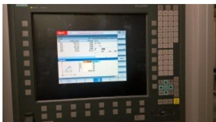
Instead of the commonly adopted separate control systems for the robot and the cleaning machine, the EcoCflex 3 relies on a single CNC controller serving both. This feature makes for simpler and faster programming, operation, maintenance, and re-starting after a part change.
