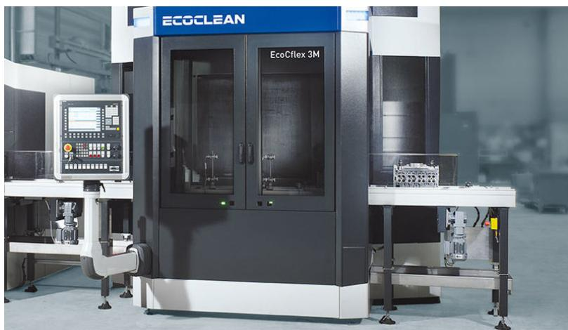
The cleaning and drying functions are separated. Drying is performed in the new EcoCdry vacuum dryer which does away with compressed air pre-drying. Part handling is thus reduced, and more treatment time is freed within the 45-second overall cycle time.
